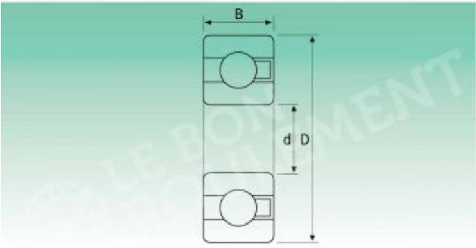
The diagram shows a cross-section of a ball bearing with dimensions labeled: B (width), d (inner diameter), and D (outer diameter).
